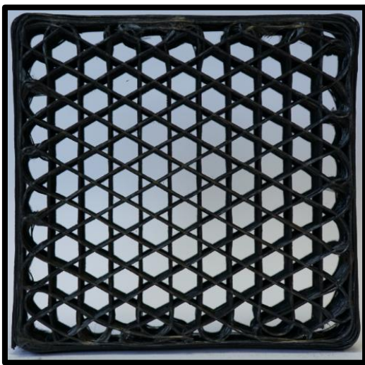
Figure 1 : structure composite C/C-SiC de type kagomé
